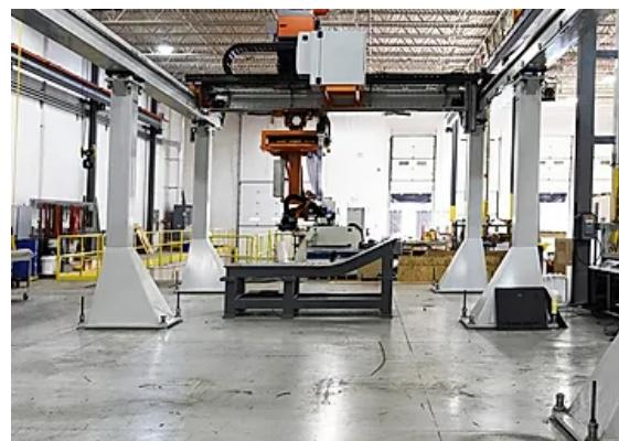
system allows for additive build sizes up to 1575" wide, 310" long and 75" tall. The ADDere SYSTEM III also has the capability to weld on both sides of a substrate to allow for the highest in additive manufacturing flexibility.
