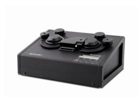
The RECOATER  $1^{\text{TM}}$  is used to restore the primary coating on spliced optical fibers with acrylate coatings. Due to the mould design, the restored part of the coating has a diameter and other properties, such as excentricity and roundness, that are almost identical to the original fiber.
